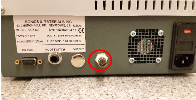
Figure 5. Back of Power supply unit where the circle indicates the socket where the Converter housing cable should be plugged in.
