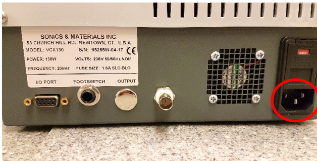
Figure 6. Back of the Power supply unit where the circle indicates the socket where the Power cable should be plugged in.
